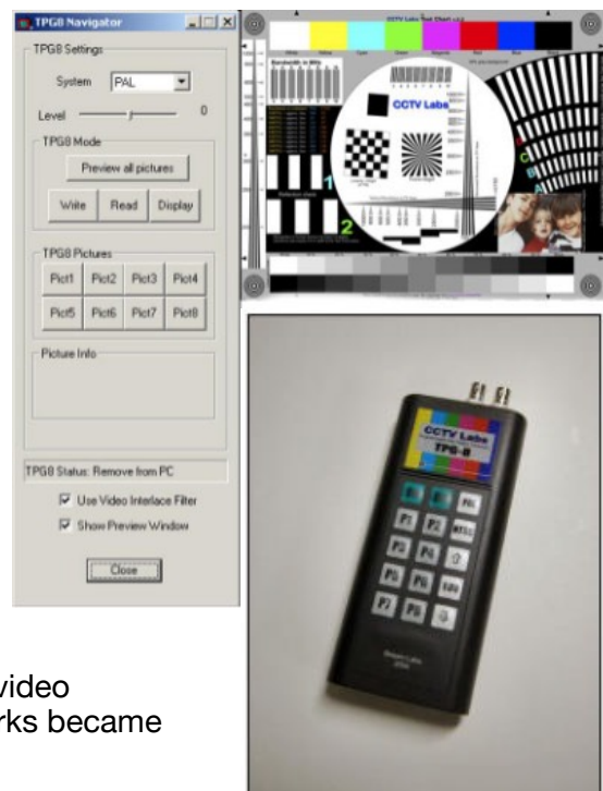
The TPG8 programmable Test Pattern Generator with the test chart v.3.0 produced electronically
