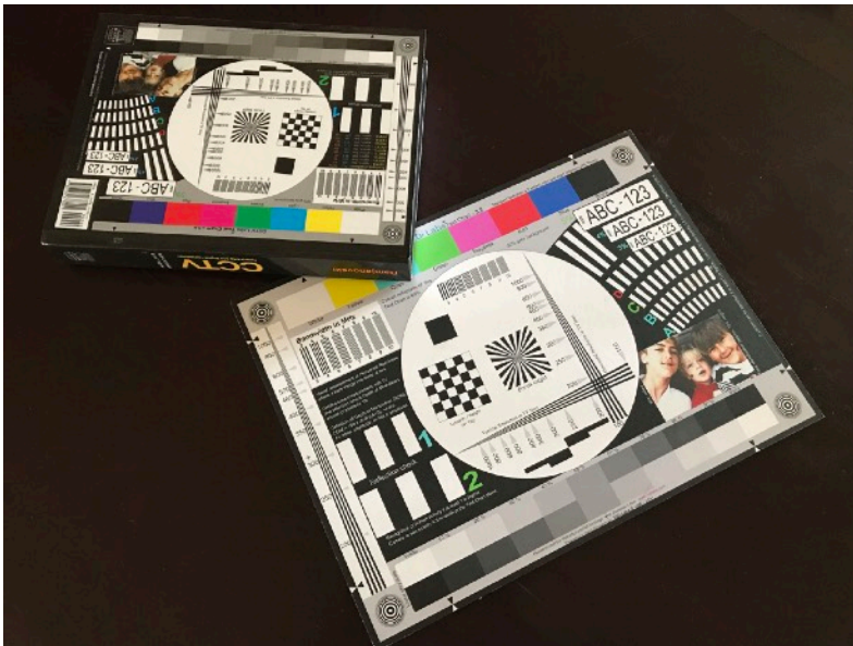
The back-cover test chart v.3.0 and a stand-alone A3 format
